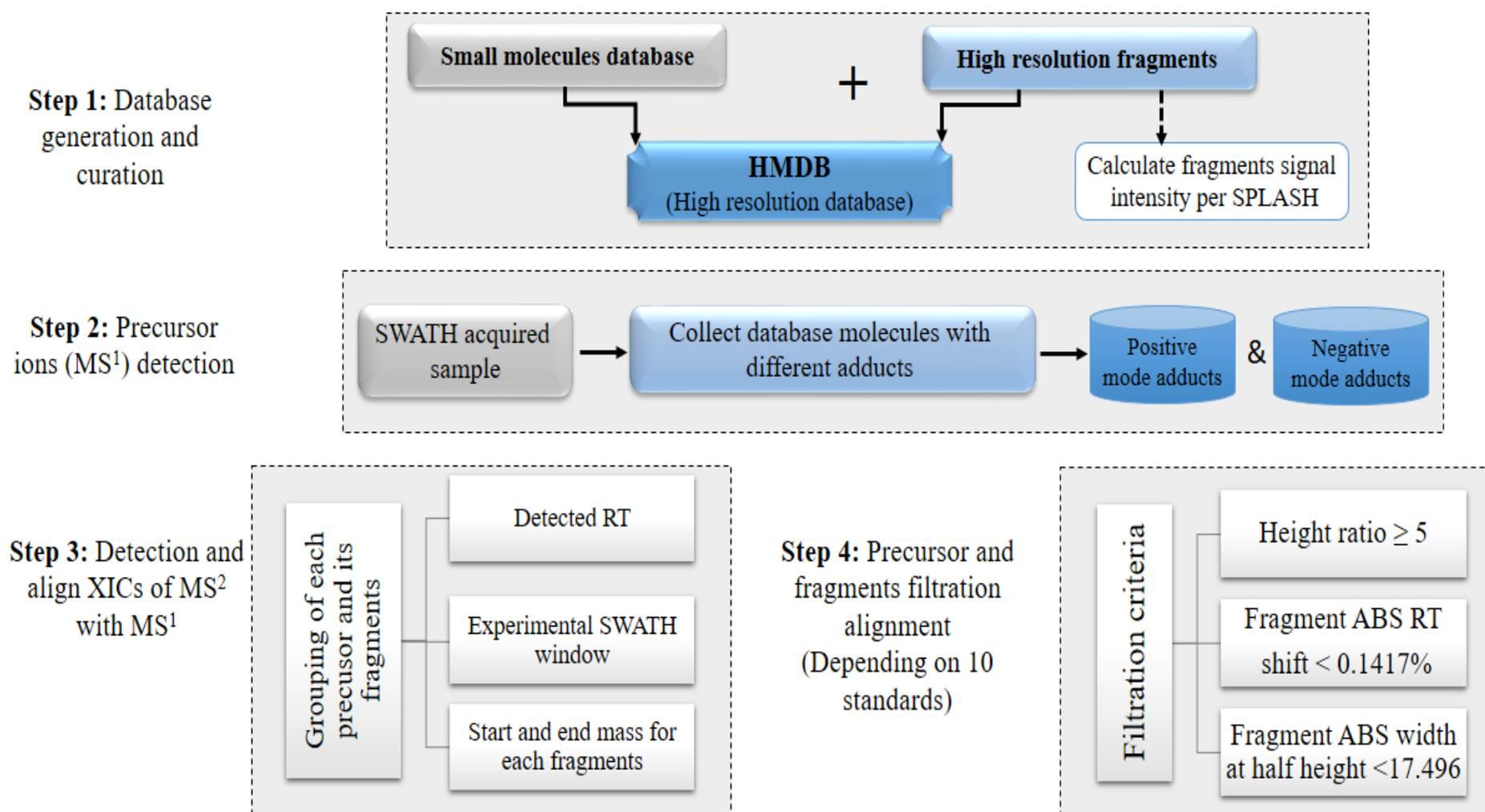
**Fig.1 Schematic illustration of SWATH-Auto System Analyzer (SASA) workflow for small molecule extraction of SWATH acquired samples.**
